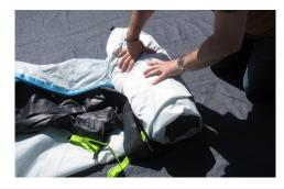
⇒ Place the rolled canopy on to the bag and pull the sides up round it. Finally, Zip up the bag.
